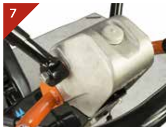
7 LARGE VOLUME OIL TANK
